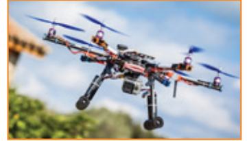
Helicopter UAVs – can hover in one place and are more controllable
