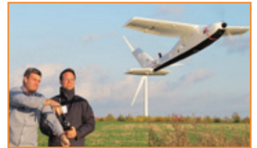
Fixed-wing UAVs – cover more distance and are able to fly in stronger winds
